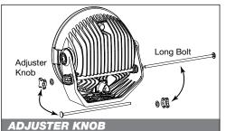
Adjuster Knob can be reversed from left hand to right hand side.
