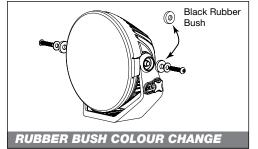
Remove the side M8 bolts, washers and blue rubber bushes. Replace with black rubber bushes. Re-assemble in reverse order.
