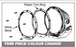
To change the colour of the Plastic Trim Ring, remove 5 x screws and Metal Bezel. Re-assemble in reverse order.
